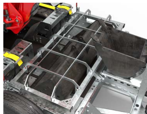
○ Bucket locker Secure lockable storage for digger buckets and other attachments.
